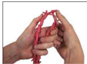
Turn belt inside out with tabs pointing outwards. Bend back as far as possible; hold with one hand. Twist one tab 90° parallel with slot.
