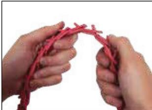
Flex belt further and insert second tab through end link by twisting tab with thumb.
